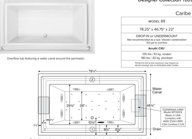
Dotted lines indicate a raised, level deck area which is optional for valves and required for whirlpool. Air bath control must be mounted adjacent to the tub and is shipped loose when ordered without deck plugs. Shown with Air Massage and Ultra Whirlpool Package.
