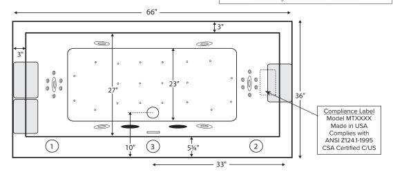
The tub features a round integrated overflow with direct toe tap drain connection directly above rough-in pipe. Numbered areas on tub deck represent possible locations to install cleaning systems, faucets and other fixtures. Shown with Air Massage and Ultra Whirlpool Package.
