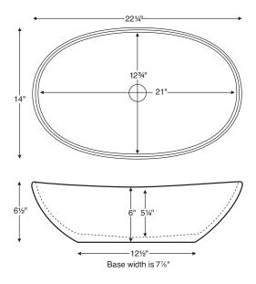
Cut-out for the drain installation required.
