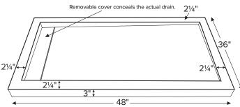
48" x 36" x 3" (exterior bottom of base) MULTIPLE, LOW-PROFILE THRESHOLD smooth floor End Drain Acrylic CXL® **DoloMatte**® 85 lbs / 39 kg 97 lbs / 44 kg
