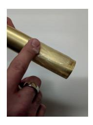
**11.** Apply provided lubricant inside the Drop-In Drain
